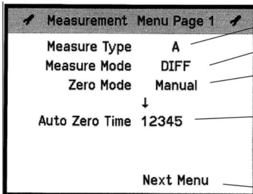
$\triangleleft$   $\triangleright$  Measure Type B,A+B,(A+B)/2,A-B,(A-B)/2, (B-A)/a
