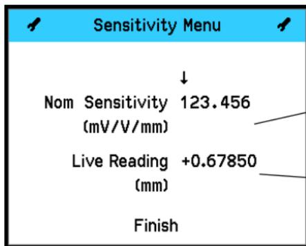
Enter Probe Sensitivity (mV/V/mm)
