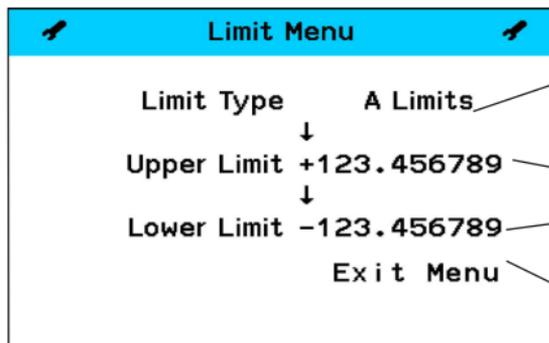
3 types of limits can be displayed A,B and "Computed Limits" when more than one measurement type selected see 6.4
